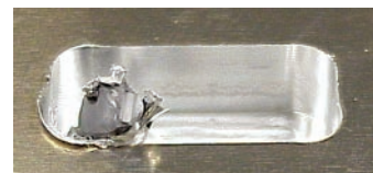
Milling with un-coated carbide end mill
