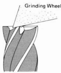
Application for Relief Angle, and Radial Rake Angle
