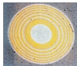
Composite multi-layer film (UG-Coating)
